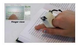
It is a ring type model that can be used for real time which is worn to the index finger. It consists of a camera that converts the text to speech. The technique of finger reader is shown in figure. The concept of optical character recognition is used in this device. Optical Character Recognition (OCR) is mechanical or electronical conversion of typed, handwritten or printed text into machine-encoded text. It widely accepts datafromanysortofdocument.
